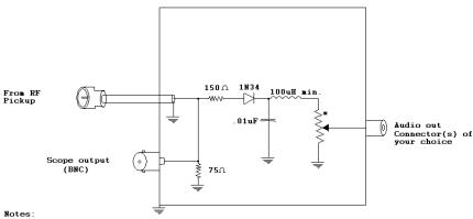
All of this is optional of course and can be made as fancy or as simple as you like. This is a minimal requirement design for clean flat response within the passband of the RF pickup, which is about -25dB from 2-50 MHz.
